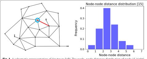
**Fig. 1** A schematic representation of Anytown (left). The node–node distance distribution of node 15 (right), highlighted in light blue in the network
