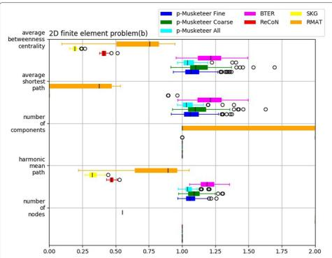
**Fig. 15** Computational results on performance of planar Musketeer 2D finite element graph with 1866 nodes and 3538 edges for number of nodes, harmonic mean path, number of components, average shortest path and average betweenness centrality
