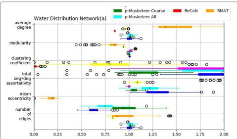
**Fig. 6** Computational results on performance of planar Musketeer on real water network with 407 nodes and 459 edges for clustering coefficient, number of edges, mean eccentricity, total degree \*degree assortativity, modularity and average degree
