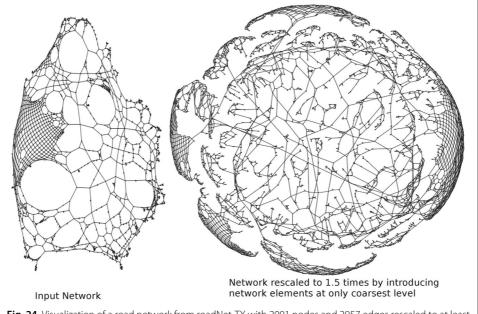
**Fig. 24** Visualization of a road network from roadNet-TX with 2001 nodes and 2957 edges rescaled to at least 5028 nodes and 7375 edges
