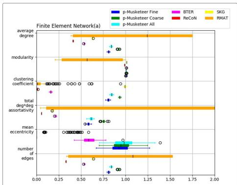
**Fig. 4** Computational results on performance of planar Musketeer on finite-element graph with 4704 nodes and 13427 edges for clustering coefficient, number of edges, mean eccentricity, total degree \*degree assortativity, modularity and average degree
