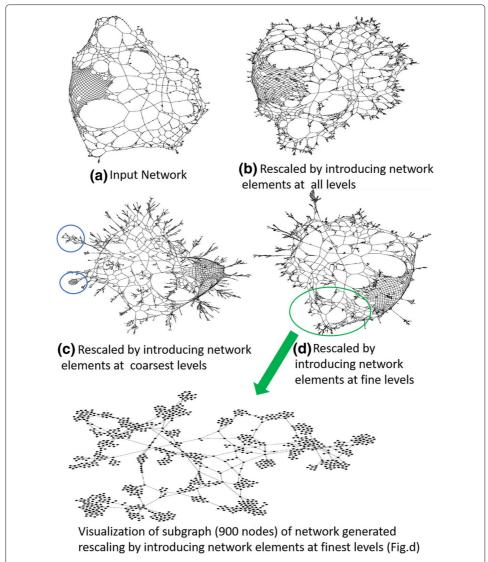
**Fig. 16** Visualization of a road network from roadNet-TX with 2001 nodes and 2957 edges rescaled to at least 5900 nodes and 7000 edges. **a** Input network. **b** Rescaled by introducing network elements at all levels. **c** Rescaled by introducing network elements at coarsest levels. **d** Rescaled by introducing network elements at fine levels
