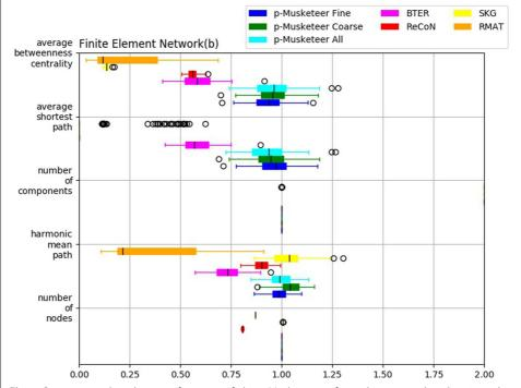
**Fig. 5** Computational results on performance of planar Musketeer on finite-element graph with 4704 nodes and 13427 edges for number of nodes, harmonic mean path, number of components, average shortest path and average betweenness centrality
