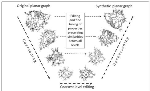
**Fig. 1** The V-model for multiscale planar network generation. The original input planar network is coarsened to generate a hierarchy of coarse networks, the process is then reversed generating fine-level networks. The number of level (here 5) depends on the size of input network or the user input
