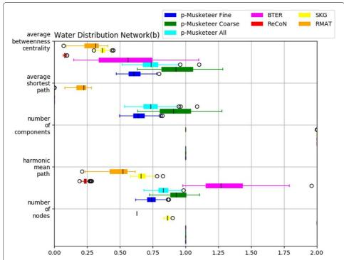
**Fig. 7** Computational results on performance of planar Musketeer on real water network with 407 nodes and 459 edges for number of nodes, harmonic mean path, number of components, average shortest path and average betweenness centrality
