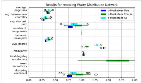
**Fig. 19** Computational results for finite-element graph with 4704 nodes and 13427 edges rescaled to at least 12700 nodes and 36000 edges
