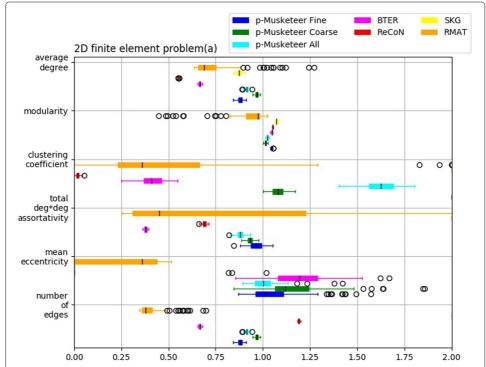
**Fig. 14** Computational results on performance of planar Musketeer 2D finite element graph with 1866 nodes and 3538 edges for clustering coefficient, number of edges, mean eccentricity, total degree \*degree assortativity, modularity and average degree
