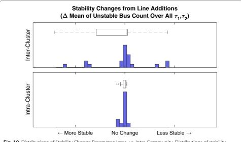
**Fig. 10** Distributions of Stability Change Parameter: Inter- vs. Intra-Community. Distributions of stability impact parameter for a) inter-community connections, and b) intra-community connections. From the histogram outliers and the spread denoted by the box plot width, it is clear that the line additions between distinct communities are much more likely to effect significant changes to network stability (positive or negative)
