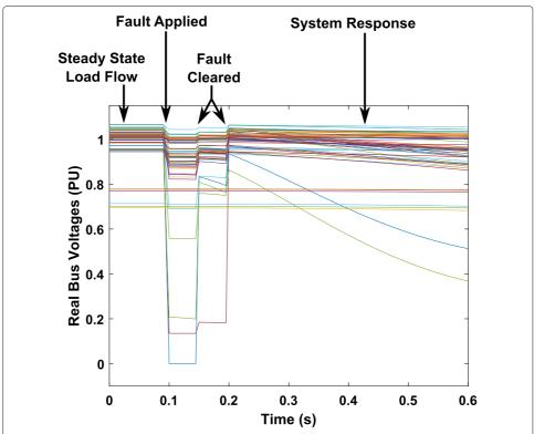
**Fig. 1** Power System Toolbox: Sample Simulation. Stages of a grid simulation in PST: The system is in a steady state until a fault is applied at 0.1s. The fault is cleared in two stages, at 0.15 and 0.2s. After the fault has been cleared, the system has been perturbed from its steady state so it continues to evolve dynamically
