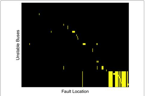
**Fig. 4** Unstable Buses Based on Fault Location. A systematic exploration of the network locations of unstable dynamics as a function of the line where the initial fault was applied. Each column represents a different simulation with a different fault location, with yellow pixels denoting which buses exhibited instability during that run
