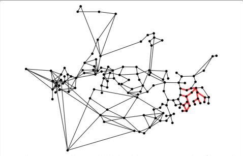
**Fig. 7** Fault Locations Susceptible to CSI. Highlighted in red: the twenty most sensitive lines of the network, i.e. those where a fault is most likely to induce CSI
