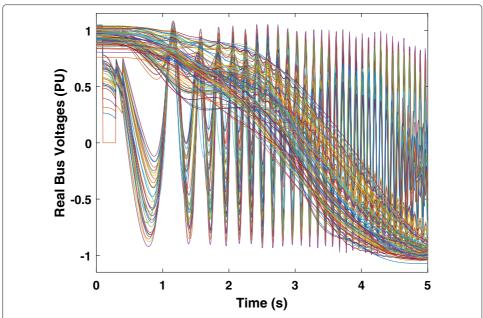
**Fig. 3** Coherent Swing Instability. CSI in numerical simulations: Plotting bus voltages shows two qualitatively different types of dynamics. Each bus belongs to one of two coherent groups, one of which varies at a slow, consistent time scale and the other of which oscillates with linearly increasing frequency
