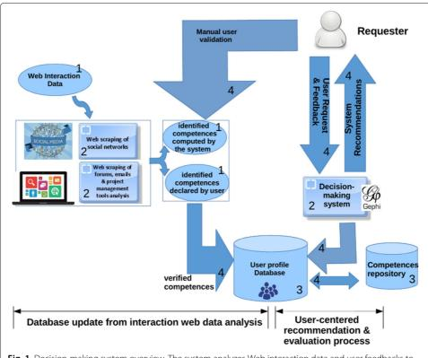
**Fig. 1** Decision-making system overview. The system analyzes Web interaction data and user feedbacks to provide the user with profile's recommendations. 1: data 2: process 3: database 4: data flow
