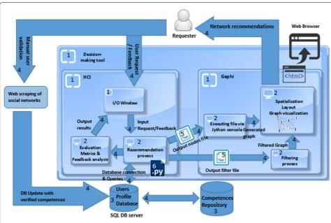
**Fig. 3** System architecture & experimental platform with two main user interfaces: Gephi for network visualization, and a developed HCl for I/O data processing. 1: user interface 2: process 3: database 4: data flow 5: text file 6: python script file
