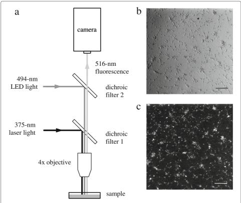
**Fig. 1 a** Schematic diagram of the apparatus. Field-of-view (FOV) **b** under Bright-field illumination and **c** of corresponding calcium indicator (Fluo-4) fluorescence. Scale bars: 200  $\mu$ m
