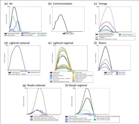
**Fig. 11** Failure behaviour of the infrastructure networks under the degree failure method. The y-axis shows the number of components and the x-axis shows the % of nodes removed from the graph, with a more robust network showing a smaller peak and towards the left of the plot
