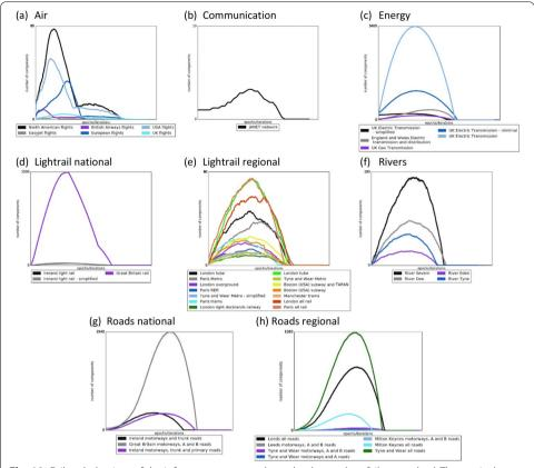
**Fig. 10** Failure behaviour of the infrastructure networks under the random failure method. The y-axis shows the number of components and the x-axis shows the % of nodes removed from the graph, with a more robust network showing a smaller peak and towards the left of the plot
