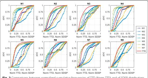
**Fig. 2** Comparisons between normalized cumulative frequencies of TTD (Norm TTD) and of SDSP distributions (Norm SDSP), based on 7 different weights, for 8 subnetworks of Dresden's sewer system (N1-N8)
