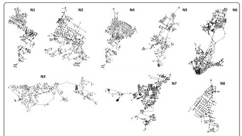
**Fig. 1** Layout for the 8 subnetworks of Dresden's sewer system (N1-N8). Red triangles identify the outlet of each network, i.e. the connections to the main wastewater collectors
