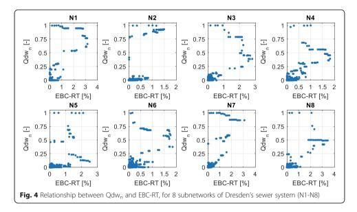
pipes with higher flows, the EBC is lower since the number of possible shortest paths decreases. This is due to the fact that, for historical and topographical reasons, destination nodes such as WWTPs are usually located on the outskirts of cities and not in the topological center, which leads to an inverse relationship between flow and EBC.
