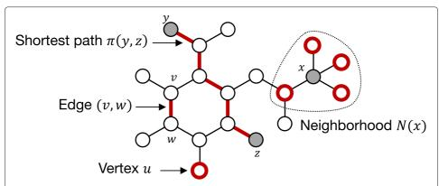
**Fig. 1** Graph representation fundamentals. Illustration of a graph G in which each circle represents a different vertex and each line connecting two circles an edge. Some edges and vertices are highlighted to illustrate specific graph concepts. Here,  $\pi(y, z)$  represents the shortest path (sequence of vertices) between vertices y and z. The neighborhood N(x) of a vertex x is the set of vertices adjacent to x
