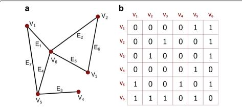
**Fig. 1 a** An example of undirected and unweighted graph G = (V, E), where V is the set of nodes and E is the set of edges. **b** The binary adjacency matrix corresponding to the graph, where zeros and ones respectively represent the absence or presence of an edge between a pair of nodes
